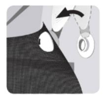
When removing your Window Shades, be sure to use the EZ Snap Removal Tool or a small flat screwdriver to separate the Fasteners.
